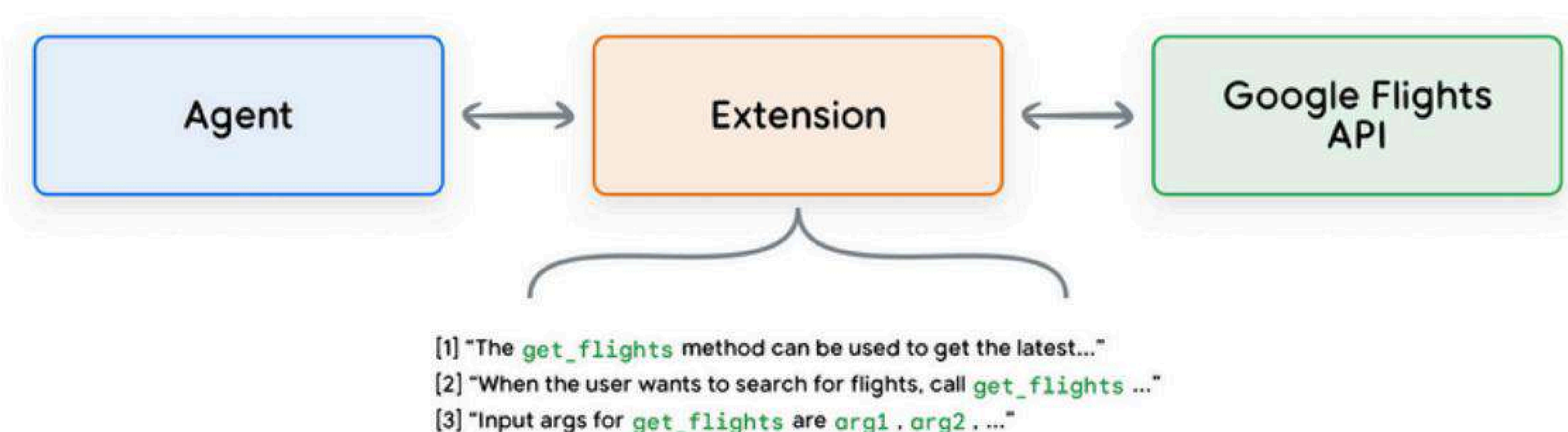
Example of an Extension connecting an Agent for flight booking to Google Flights API
